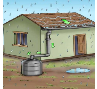
Rain Water Harvesting and other storage units
